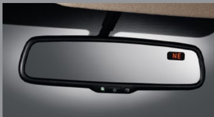
Auto-dimming Rearview Mirror with Compass
