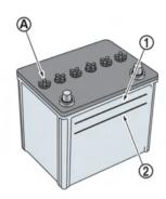
Check the fluid level in each cell (Remove the battery cover if it is necessary). It should be between the UPPER LEVEL (1) and LOWER LEVEL 2 lines.
