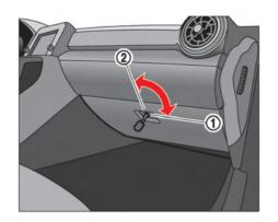
Use the mechanical key to lock 1 and unlock 2 the glove box. (  $\nearrow$  "Mechanical key" page 3-3)
