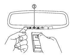
2. Using both hands, simultaneously press and hold the desired HomeLink® button and handheld transmitter button. DO NOT release until the HomeLink® indicator light ① flashes slowly and then rapidly. When the indicator light flashes rapidly, both buttons may be released. (The rapid flashing indicates successful programming.)
