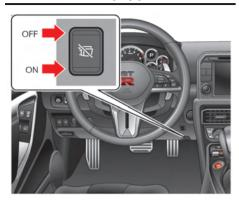
The exhaust sound control switch on the lower side of the instrument panel allows the driver to turn the exhaust sound control system on and off.
