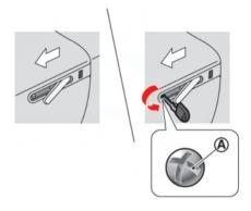
2. With the outside door handle lifted up. use the mechanical key and turn the key cylinder cap (A) counterclockwise to remove.
