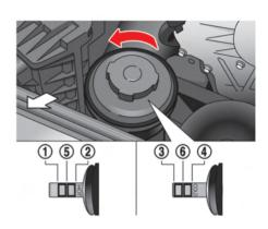
NISSAN recommends to adjust the engine oil level ① to be 0.39 in (10 mm) (1/8 gal (0.5 liters)) ② below the H mark on the engine oil dipstick. (③ range is 1.18 in (30 mm).) Before checking the oil level, run the engine until it reaches operating temperature and wait at least 5 minutes after turning off the engine. Make sure the oil level always remains above the L mark.
