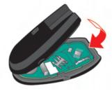
Reconnect the upper and lower parts of the Intelligent Key.
