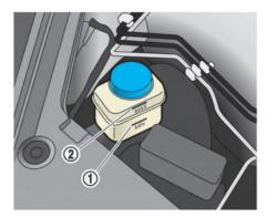
Check the fluid level in the reservoir. If the fluid is below the MIN line ① or the brake warning light comes on, add Genuine NISSAN Brake Fluid R35 Special II fluid (or equivalent) up to the MAX line 2. If fluid must be added frequently, the system should be checked. It is recommended vou contact a GT-R certified NISSAN dealer.
