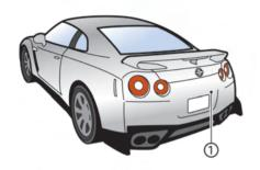
If dirt, rain or snow accumulates on the camera (1), the RearView Monitor may not display objects clearly. Clean the camera by wiping it with a cloth dampened with a diluted mild cleaning agent and then wiping it with a dry cloth.
