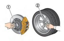
5. Remove the wheel nuts and then remove the wheel.
