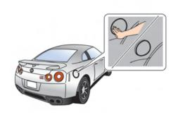
2. Press the rear side of the fuel-filler door to release the door lock, and open the door.
