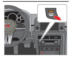
To defog/defrost the rear window, start the engine and push the switch on. The indicator light on the switch will come on. Push the switch again to turn the defroster off.
