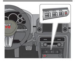
The control of the dual clutch transmission, Bilstein DampTronic® electronically controlled shock absorbers and Vehicle Dynamic Control (VDC) can be changed to the desired modes by operating the setup switches. Select the desired mode best suited to the driving conditions.
