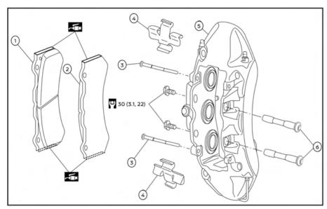
1. Inner pad (with pad wear sensor)
