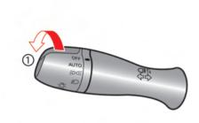
The autolight system can turn on the headlights automatically when it is dark and turn off the headlights when it is light.
