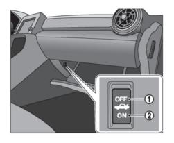
valet and keep the mechanical key with you. ( The "Valet hand-off" page 3-3) To connect the power to the trunk lid, push the switch to the ON position 2.
