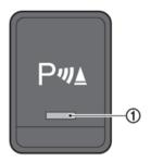
The sonar system OFF switch on the lower side of the instrument panel allows the driver to turn the sonar system on and off. To turn the sonar system on and off, the ignition switch must be in the ON position. The indicator light 1 on the switch will turn off when the system is turned off. If the indicator light flashes it may indicate a malfunction in the sonar system.
