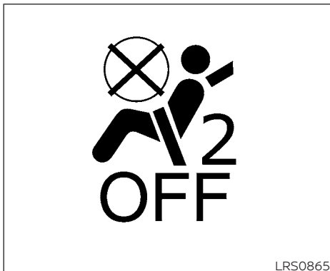
Front passenger air bag and status light
