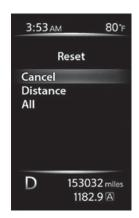
Drive computer 2 will automatically reset each time the ignition is placed in the OFF position.
