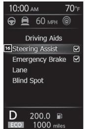
Steering Assist may not operate as expected under all conditions. Always be prepared to steer if needed. For example, lighting conditions, weather, lane splits (such as exit ramps) and confusing lane markers may cause the system to not
