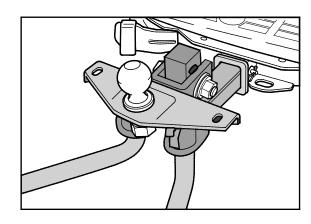
weight-distributing hitch ball mount (Class IV) is recommended if you plan to tow trailers with a maximum weight over 5,000 lbs. This ball mount includes a 2-5/16" hitch ball and is available through your NISSAN dealer.
