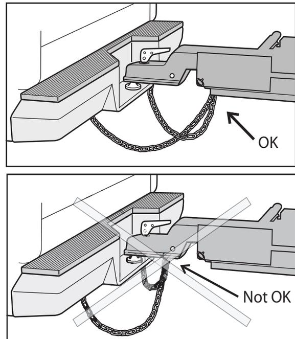
**⚠ WARNING- DO NOT** use S-hooks for attaching the safety chains as they may become un-hooked while towing. If the S-hook unhooks, the emergency chains/cables will become detached, so if the tow hitch breaks or becomes disengaged, it will allow the trailer to completely break away causing property damage and possibly personal injury or death. The use of S-hooks is illegal in many states.
