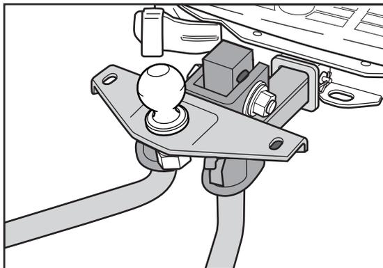
**Clamp-On Bumper Hitch** - This temporary hitch clamps onto the bumper assembly.
