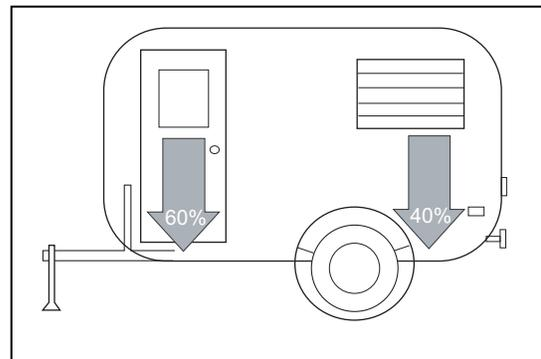
With this in mind, proper loading is extremely important. When loading a trailer, 60% of the total cargo weight should be positioned in the front portion of the trailer and 40% in the back. Then, adjust the load until the proper tongue/king pin load ratio is achieved.
